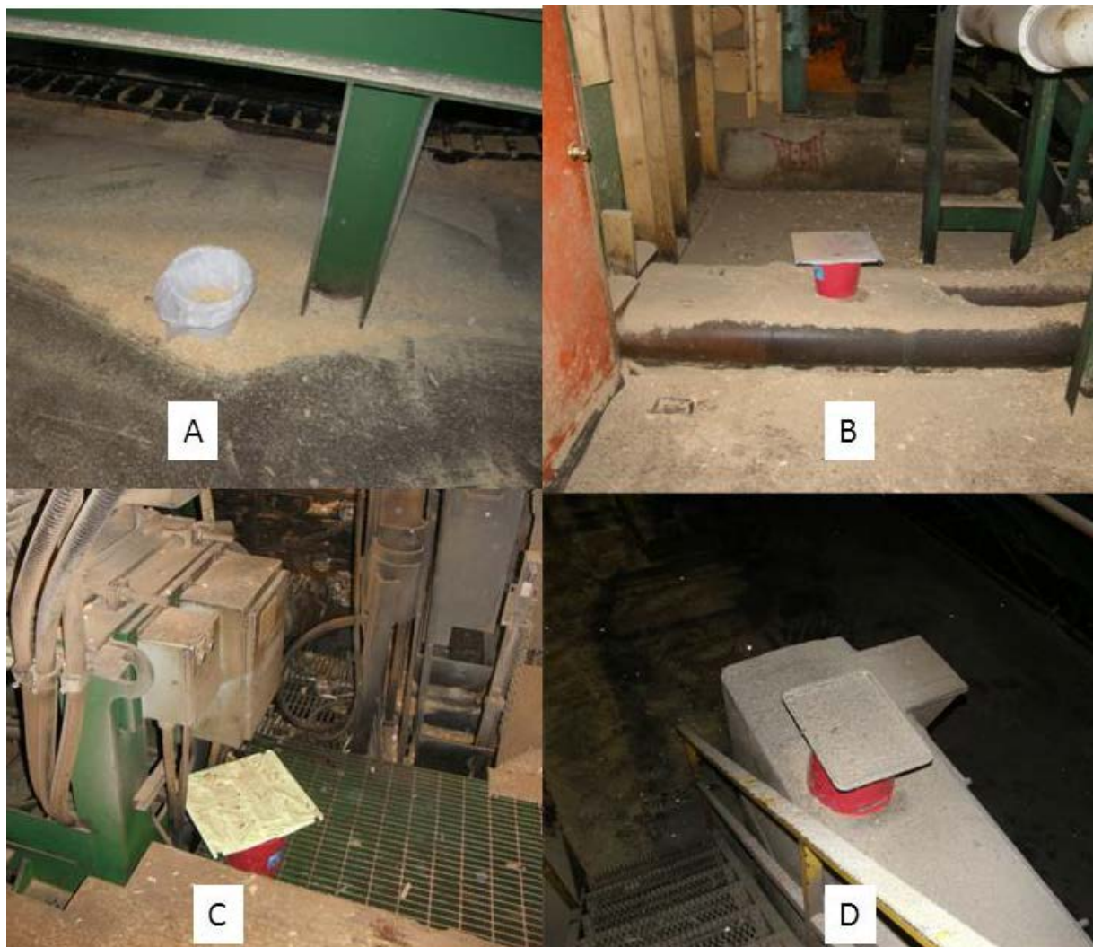
Figure 2 Four types of receptacles were deployed to sample sawmill dust as it was generated: A) bucket lined with a plastic bag, B) tray covered with parchment paper, C) tray covered with microfibre cloth and D) an unlined tray (C and D were less effective and used only in the first two mills)
