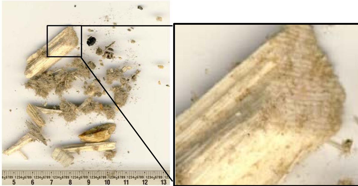
Figure 7 Particles retained by the 1000µm sieve with clumps of fine material adhering to the larger particles
